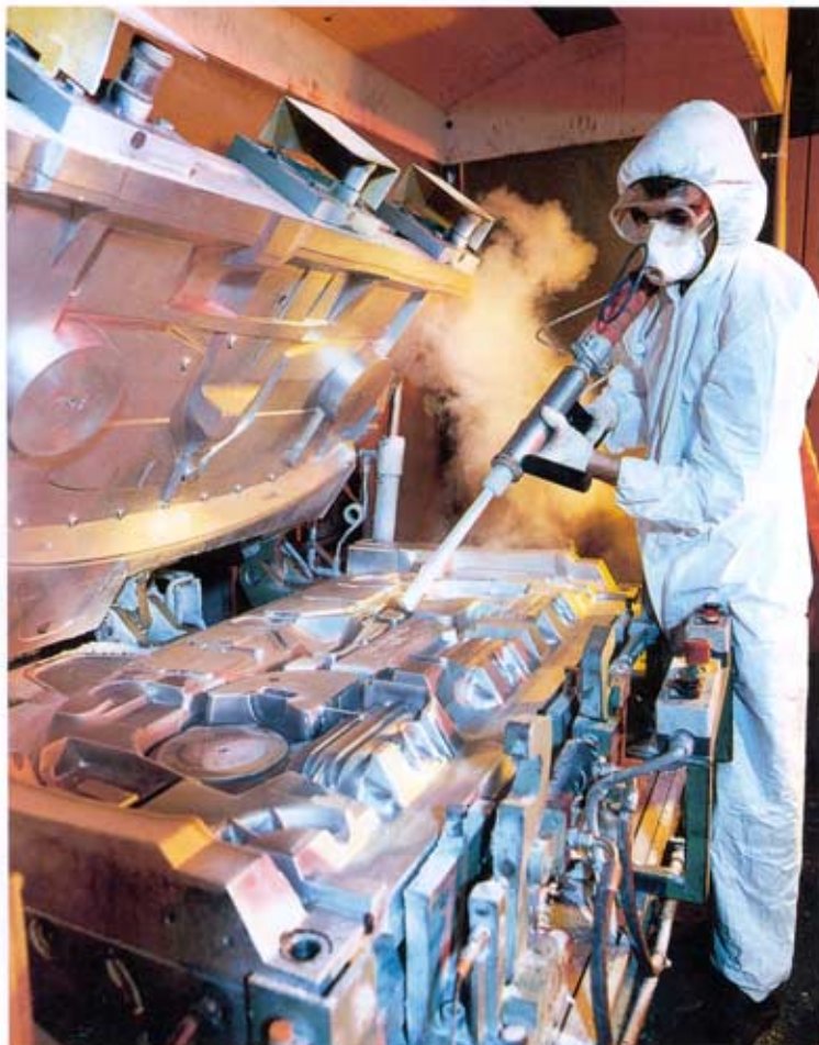
A genuine alternative to known cleaning methods: The CO 2 blasting process.
